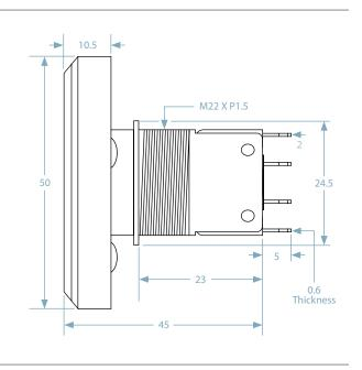
You can touch the push button on any part of the face to create the contact action.
